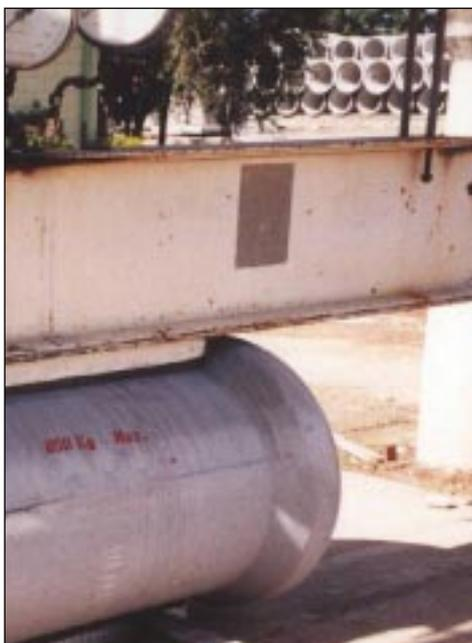
The pipe load class is determined by this physical testing procedure and is the point of interface between the manufacturing process and the calculated load on a pipe for a specified bedding installation.
