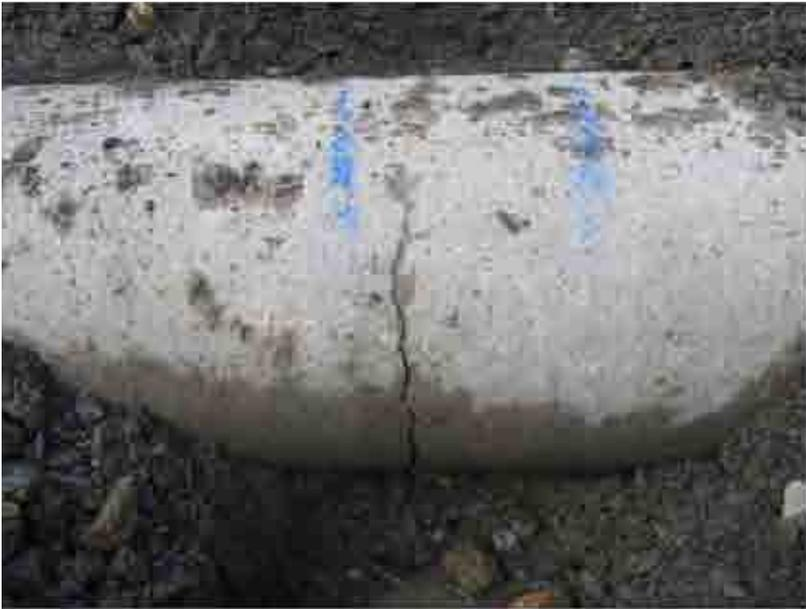
*A 6mm crack at the bottom of a DN300 pipe due to stresses resulting from poor bedding.*
