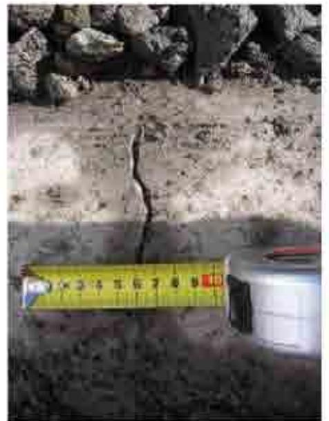
*A 6mm crack at the top of a DN300 pipe due to stresses that have resulted from poor bedding*
