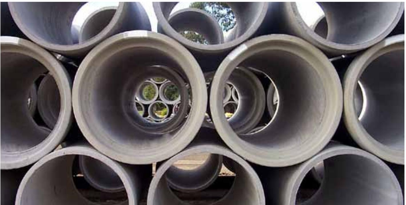
*Typical Smooth Bore of Concrete Pipe.*
