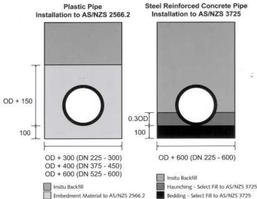
Fig.8 - Embedment geometry comparison.
