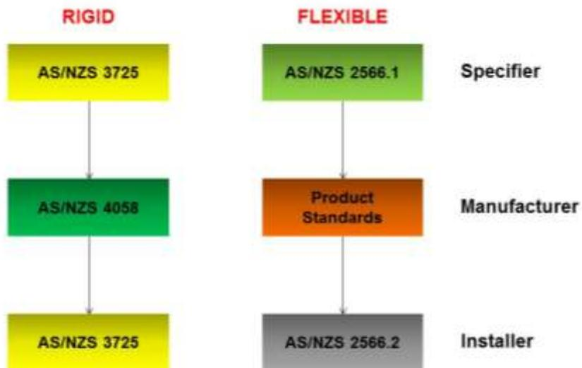
Figure 1 - Australian/New Zealand Standards for Pipe Design & Installation
