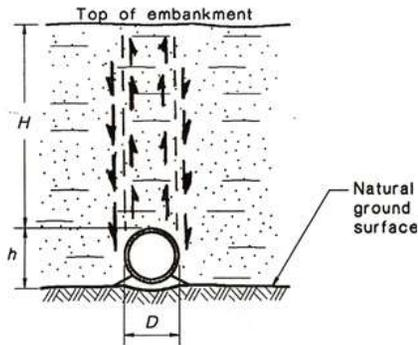
Fig.3 - Embankment fill load  $W_g = C_e w D H$
