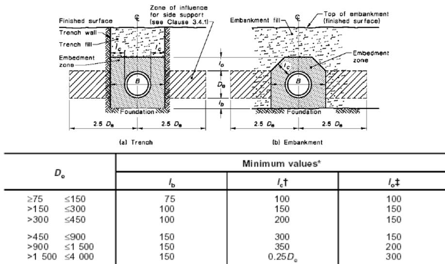
Fig.7 - Flexible pipe embedment geometry (Ref. Excerpt AS/NZS 2566.1 Fig.3.1)
