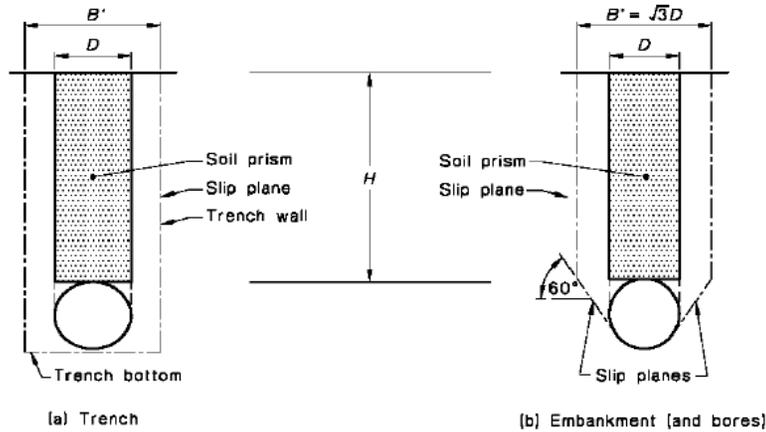
Fig.6 - Soil Prism Load - Flexible Pipe (Ref. AS2566.1 Fig.C4.1)
