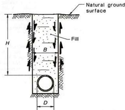
Fig.2 - Trench fill load  $W_g = C_t w B^2$
