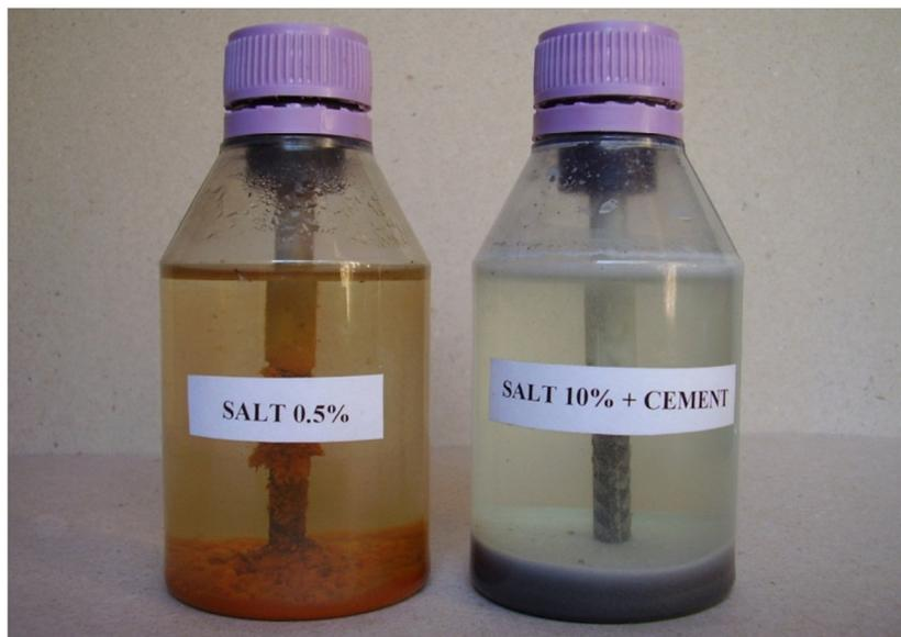
Figure 2. Samples of reinforcing steel in salt solution
