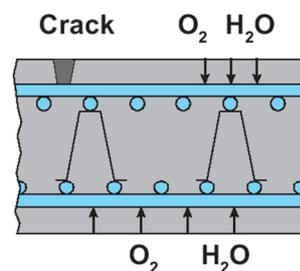
$$\text{Rate of corrosion} = f(\text{O}_2, \text{H}_2\text{O at Cathode}) / (\text{Resistivity of Concrete})(\text{Size of Cathode})$$
