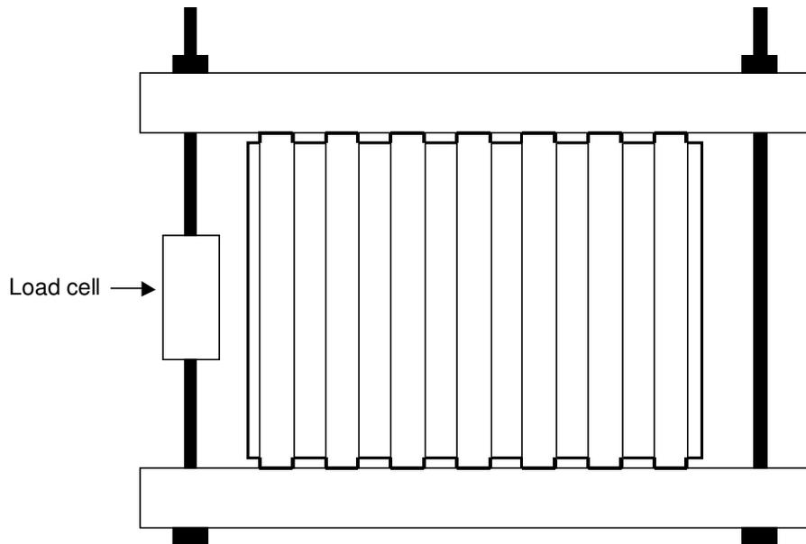
Total applied load is twice the reading from the load cell
