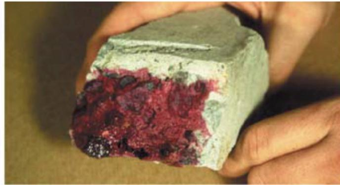
Typical effect with concrete of average quality – significant depth of carbonation within the service life
