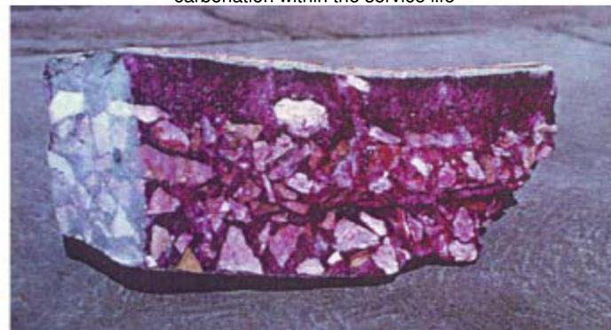
Concrete pipe made in the early 1920s, not installed but exposed to the weather for 65 years (wall thickness 75mm)
